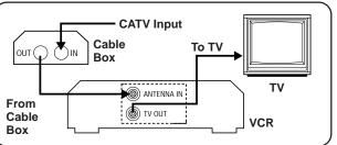
With this connection you can view/record any cable channel <u>including scrambled channels to which you have subscribed.</u>
